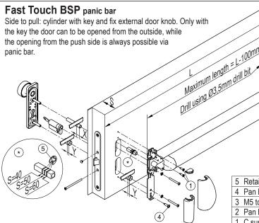
S=60mm Y= 0mm X= 0mm S=50mm Y= 5mm X=10mm S=40mm Y=10mm X=20mm
