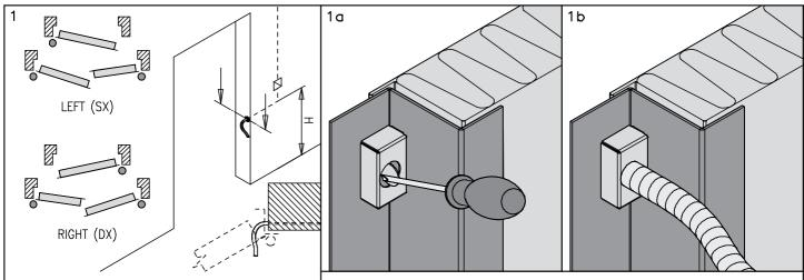
Verify and ascertain the opening direction of door. Verify the position of the power source tube. The sketch shows the opening of a right—handed door. H standard aprox. 850 mm.
