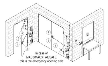
Both MAC and MAC FAILSAFE access control system can be installed onto one-leaved doors or on the main leaf of two-leaved doors in REVER, UNIVER or PROGET versions.
