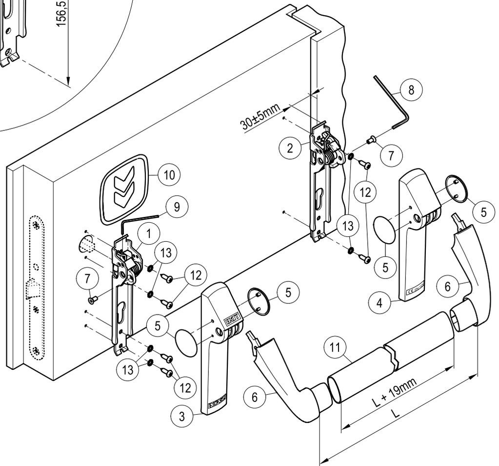
**CONTENTS OF THE "TWIST PANIC EXIT DEVICE - SPARE BAR SET + BAR" PANIC DEVICE PACKAGE**
