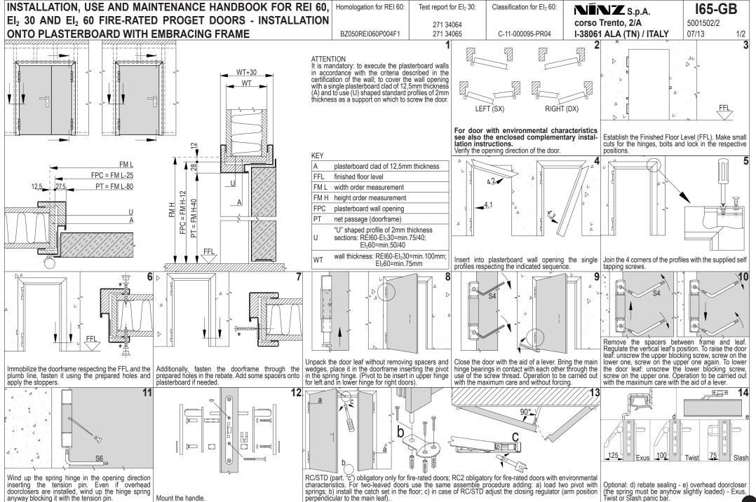
\* screws to be used (not supplied): REI= drywall screws Ø3.5x35mm; El<sub>2</sub> 30= drywall screws Ø3.5x45mm; El<sub>2</sub> 60= self-tapping screws Ø5.5x32mm
