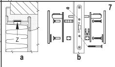
Fill up the space between doorframe and wall with mortar, without bending the frame, cover the frame with plaster and check the leeway.
