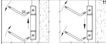
Adjusting of the ball-bearing hinges
