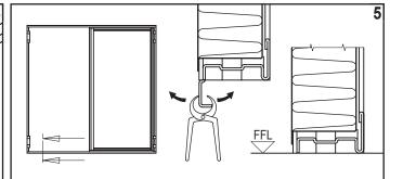
Once established the finished floor level (FFL) and decided that the door will be leaned without bottom frame, cut the jutting out fin of the lower transom so to lay the profile correctly on the finished floor level.
