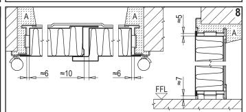
Fill up the space between the doorframe and the wall with mortar (detail A) without bending the doorframe and covering it with plaster. Remove the angle bars (part. 4b - draw. 4) to set free the inactive leaf. It is imperative to retighten both screws (4a) at top and bottom of inactive leaf. Check the leeway
