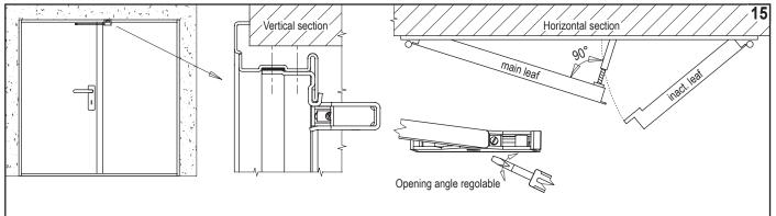
Apply the bracket and the closing regulator following the handbook included in the RC/STD kit delivered with the door equipment.
