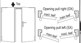
As standard the fire-rated door will be delivered from the factory with opening pull DX (right). To change the opening pull in SX (left) follow the next easy instructions.
