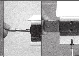
Remove the lower rod and the respective angle bar.
