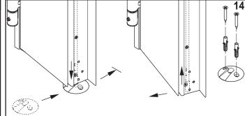
Install without lower rebate, position the floor catch beneath the passive leaf, close it and insert the lower rod into the floor catch. Open the leaf without moving the floor catch and fix it to the floor with screws and plugs.
