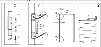
Fix the hinge frame on the secondary leaf putting in the pin for the spring hinge (X) and screwing on without overtighten both the socket set screws of the ball bearing hinge (Y). Perform the operation very carefully. Insert on the top and bottom the two spacers (Z) in equipment.
