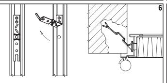
Bend up the frame-brackets and mark on the wall their positions respecting the FFL level. Create the holes in the wall for the brackets.
