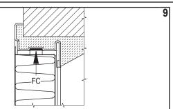
Remove all the plastic spacers between doorframe and leaf. Apply the thermo expanding gasket (FC) on the upper transom, but cut it before in two pieces with a measure that is going from the roller insert to the opposite angle of the doorframe.
