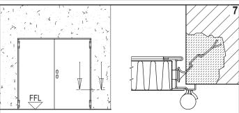
Install the principal door leaf and check that the two leafs are positioned at the same height (see point 2). Temporarily immobilize the door in the wall space, using a FFL level, true to the wall, the finished floor and the parallel walls and fix the wall anchors with quick drying cement.
