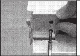
Screw again the upper and lower external plates (M5 screw on device side).
