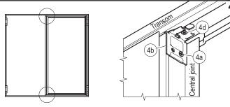
To make easier the following operation, release the prefixed screws (4a) of the angle bars (4b) placed at top and bottom of the central joint. Fix the two transoms to the inactive leaf and screw them with the screws (4d) in equipment with the handle box. Fix very well all screws.
