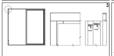
Join together the two transoms and the other hinge doorframe with the fixing flaps. Bend the flaps on the four corners to block the frame.
