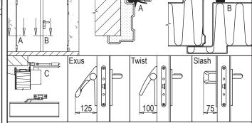
Accessories: A, B= rebate sealing - C= overhead door closer (the spring hinge must be anyhow slightly loaded) - EXUS, TWIST or SLASH panic bar.
