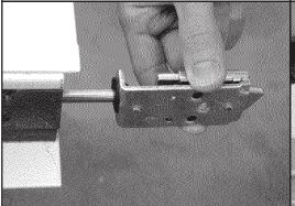
Remove the upper rod, the upper device and the respective angle bar.
