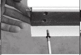
Screw the upper device with its own angle bar with the screw M5.
