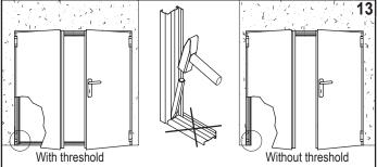
Warning: the threshold does not be removed in case of door with environmental characteristics.
