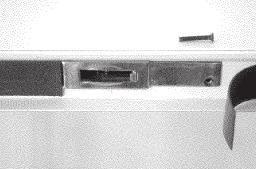
Screw the lock (M6 screw) and stick again the thermo Screw again the upper 10 expanding gasket FC, add if necessary two drops of silicone.
