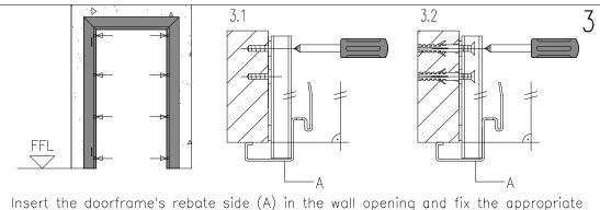
brackets with the supplied screws  $(4.8 \times 50)$  or with  $\phi$ 6 plastic anchor, respecting
