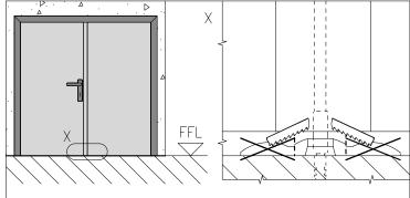
Use the same assembling procedure for the standard two leaved doors. Fasten with screw/plastic anchor and one drop of silicon the floor catch set for the lower rod of the secondary leaf and cut the four unneeded guides.
