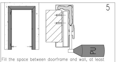
near the floor, with polyurethane foam, avoiding every deformation of the doorframe.
