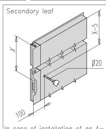
In case of installation of an Atype panic bar onto the secondary leaf, drill the first metal sheet on the indicated position.
