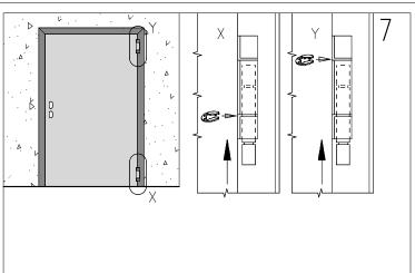
Apply the leaf by inserting the two pivots in the hinges and block them with the supplied retaining rings. Perform this operation very carefully.
