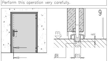
In case of Rever "Secur" door, plug the floor cathc set to the floor.
