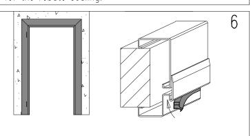
Remove the residual foam and insert the rebate sealing into the groove of the doorframe.
