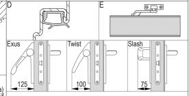
Optional: D) rebate sealing - E) overhead doorcloser (the spring must be anyhow slightly loaded) - Exus, Twist or Slash panic bar
